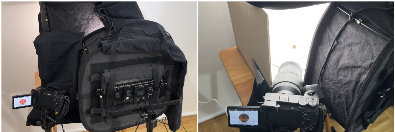
Fig. S8. Behind the scenes of our material acquisition system (Figs. 16, S7): We capture small material samples (marbles with approximately 16 mm diameter) on a motorized turntable using a single camera (Sony Alpha 6700 camera with a Sony E PZ 18–200 mm F3.5–6.3 OSS lens). The marbles are placed inside a custom-built light box made from white-laminated fiberboard, providing controlled and uniform illumination using two LED video lights (Neewer NL660-2.4G) equipped with softboxes and set to a correlated color temperature of 4400 K.
